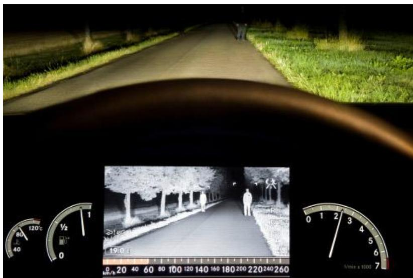
**Figure 11.** Thermal cameras can detect not only pedestrian but also wildlife on or close to roads. Source: <http://www.techconnected.com/wp-content/uploads/2013/11/Night-Vision.jpg>
