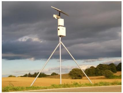
*Figure 10*. A detail of the system, based on acoustic warning of ungulates, developed during the LIFE-STRADE project. See the loudspeakers from which voice of humans and dogs barging is emitted. Photo: M. Bíl (CDV).
