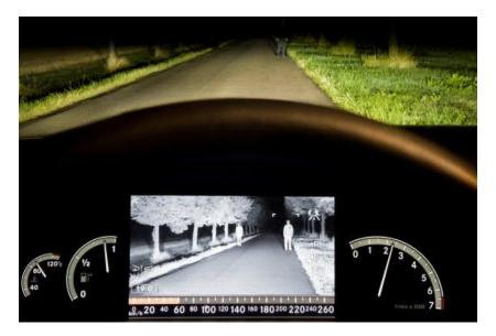
**Figure 11.** Thermal cameras can detect not only pedestrian but also wildlife on or close to roads. Source: <u>http://www.technected.com/wp-content/uploads/2013/11/Night-Vision.jpg</u>
