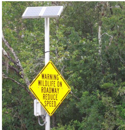
Figure 8. A text-based RADS warning sign in Big Cypress National Preserve, Florida, USA. When an animal is detected near the road, the lights begin to flash. Credit: Molly Grace
