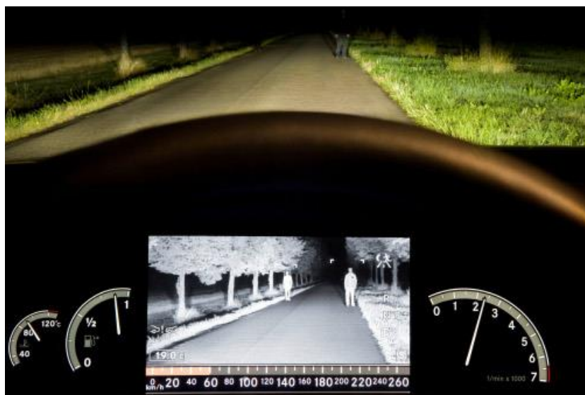
Figure 11. Thermal cameras can detect not only pedestrian but also wildlife on or close to roads. Source: http://www.technected.com/wp-content/uploads/2013/11/Night-Vision.jpg
