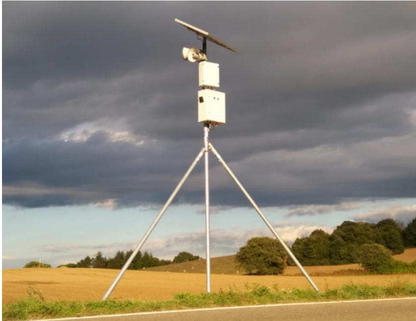
Figure 10. A detail of the system, based on acoustic warning of ungulates, developed during the LIFE-STRADE project. See the loudspeakers from which voice of humans and dogs barking is emitted. Photo: M. Bíl (CDV).
